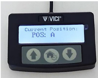
Figure 4. Manual remote control for valve actuator showing the actual valve position.
